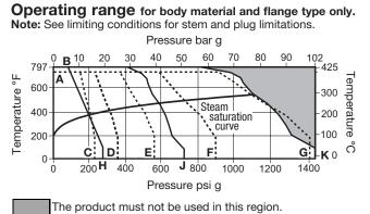
A-C PN16, A-D PN25, A-F PN63, A-G PN100 A-E PN40, **B-H** ASME 150, **B-J** ASME 300, **B-K** ASME 600
